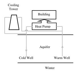
Fig. 2. Combination of ATES with a heat pump for heating and cooling of the buildings
