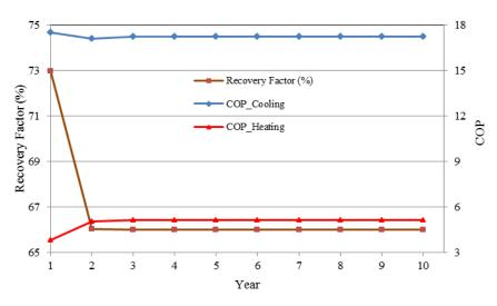
Fig.7. The Recovery Factor of the Aquifer and COP in the ATES Coupled with a Heat Pump, for Ten Years of Operation
