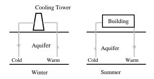
Fig. 1. Cooling through ATES alone
