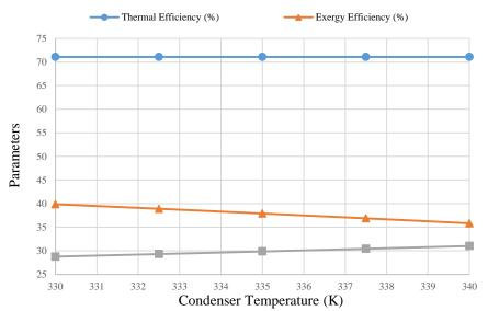
**Fig. 5.** Effect of the condenser temperature on thermal efficiency, exergy efficiency, and overall exergy destruction ratio
