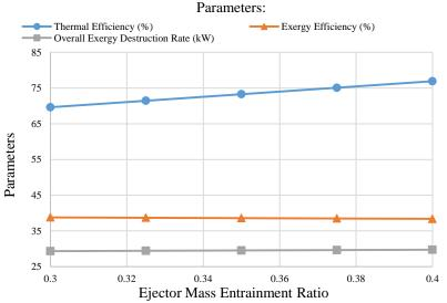
**Fig. 4.**Effect of the ejector mass entrainment ratio on the thermal efficiency , exergy efficiency, and overall exergy destruction ratio
