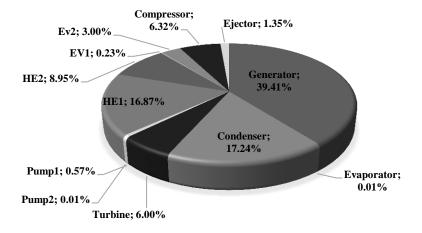
Fig. 6. Contribution of each component on the irreversibility of the proposed CCHP system
