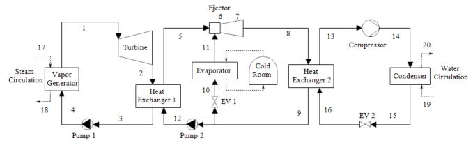
Fig. 1 Schematic of thermodynamic cycle of the proposed CCHP system
