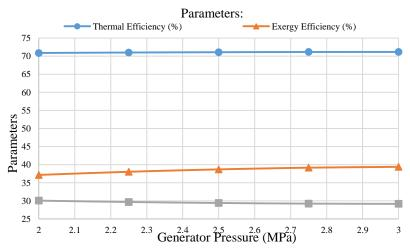
**Fig. 2.** Effect of the generator pressure on the thermal efficiency, exergy efficiency, and overall exergy destruction ratio
