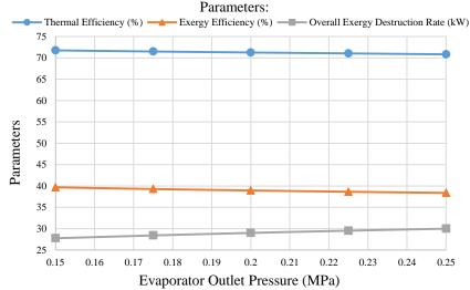
**Fig. 3.** Effect of the evaporator outlet pressure on the thermal efficiency, exergy efficiency, and overall exergy destruction ratio
