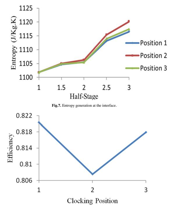
Fig.8. Efficiency of the clocking position.
