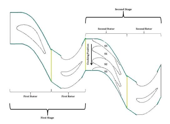
Fig. 1. Two-stage configuration of the investigated turbine
