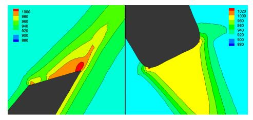
Fig.3. Entropy generation at the trailing edge of the rotor (left) and the stator (right).
