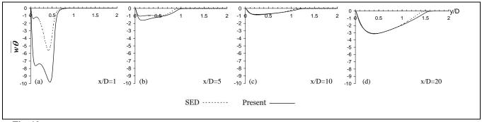
Fig. 10. Spanwise turbulent heat flux distributions at the center-line plane: comparison of SED with the present first-moment closure.
