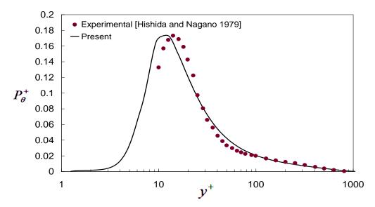
Fig.6. Variations of production of the normalized temperature variance
