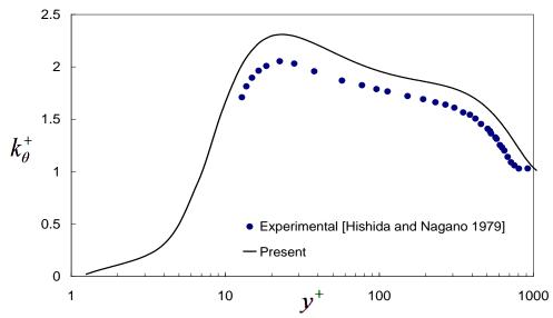
Fig.5. Profiles of normalized temperature variance in wall coordinates
