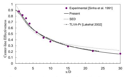
Fig. 7. Streamwise variations of Center-line film cooling effectiveness.
