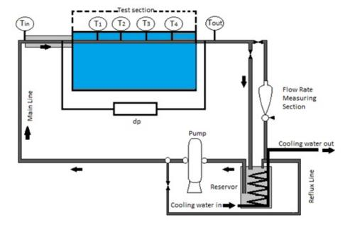
Fig. 1. Schematic of the test apparatus
