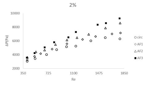
Fig. 10. pressure drop of nanofluid 2% in tubes
