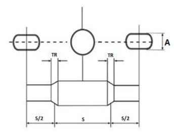
Fig. 4. Schematic of alternating flattened tube
