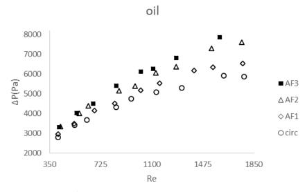
Fig. 6. pressure drop of the Base oil in tubes
