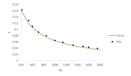
Fig. 3. Comparison of the pressure drop results from the test apparatus with the Darcy equation
