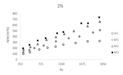
Fig. 8. heat transfer of nanofluid 2% in tubes
