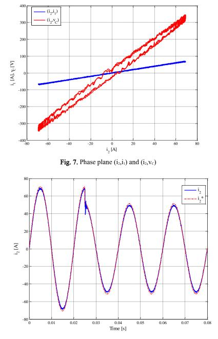
Fig.8. Grid-side current during a step change in reference power
