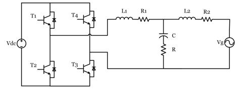
**Fig.1.** Schematic of LCL-based grid-connected inverter **Table 1.** Feasible switching states of the inverter
