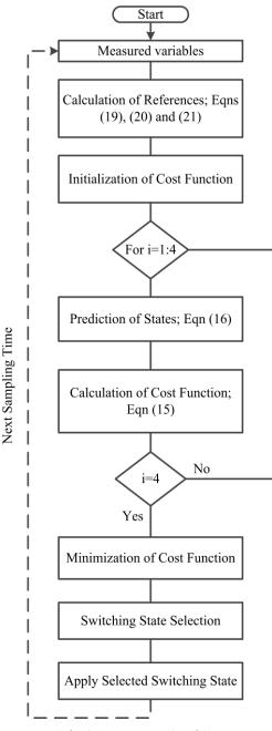
Fig.4. FCS-MPC algorithm
