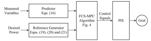
Fig.3. Proposed control scheme for PIS
