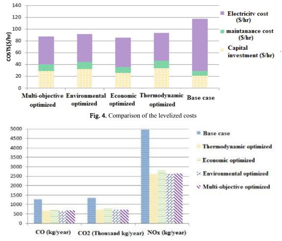
Fig. 5. Comparison of emission product for various designs of the compression refrigeration system
