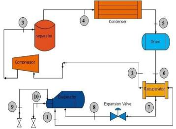
Fig. 1. Schematic arrangement of a vapour compression refrigeration system
