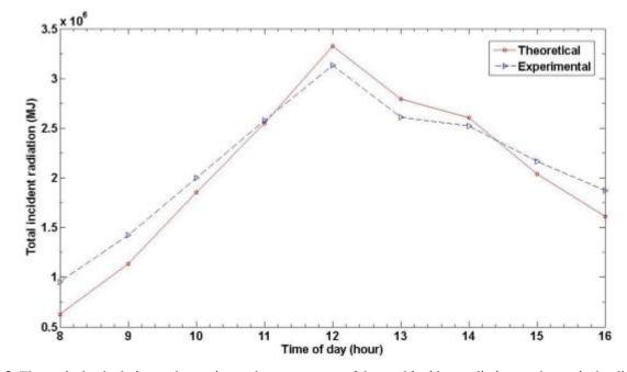
Fig. 8. Theoretical calculation and experimental measurement of the total incident radiation on the conical collector
