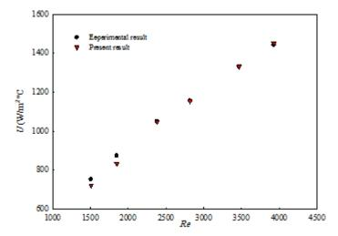
Fig. 7. Comparison between the measured overall heat transfer coefficient and simulated values using distilled-water
