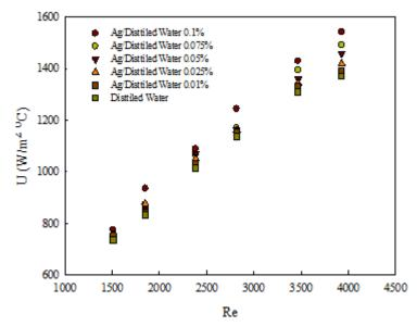
Fig. 11. Overall heat transfer coefficient of distilled-water/silver nanofluid compared to Reynolds number for different volume fractions of particles
