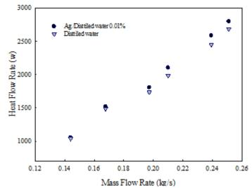
**Fig. 9.** Comparison of the heat transfer rate between the distilled-water and distilled-water/silver nanofluid with volume fraction of 0.01% at different flow rates
