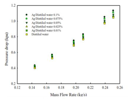
**Fig. 14.** Comparison of the pressure drop of distilled-water with silver nanofluid, with volume fractions of 0.01%, 0.025%, 0.05%, 0.075% and 0.1% at various temperatures and flow rates
