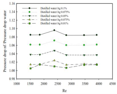
Fig. 15. The pressure drop ratio of distilled-water/silver nanofluid to distilled water
