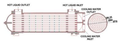
Fig. 5. Schematic of shell and tube heat exchanger with a shell pass and two tube passes
