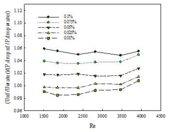
Fig. 16. Performance Index of distilled-water/silver nanofluid compared to pure distilled-water
