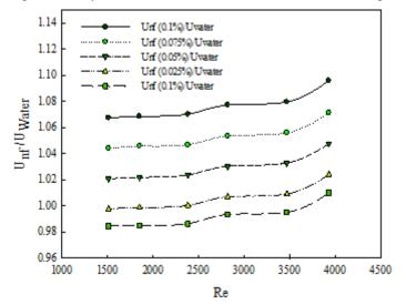
Fig. 12. Increase ratio of overall heat transfer of nanofluid and distilled water
