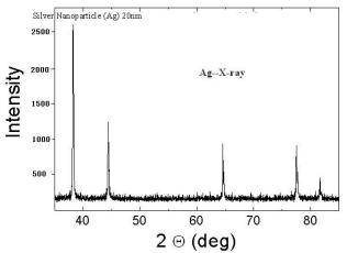
Fig. 1. X-ray of silver nanoparticles of 20 nm in diameter
