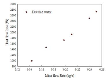
Fig. 6. The heat transfer rate of distilled-water/distilled-water
