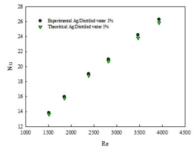
**Fig. 8.** Comparison of experimental and calculated values of Nusselt number against Reynolds number for distilled-water/silver nanofluid with a volume fraction of 0.1%
