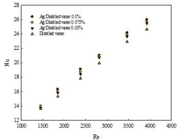
**Fig. 13.** Comparison of the Nusselt number with Reynolds number at different temperatures of base fluid and nanofluid, with volume fractions of 0.1%, 0.075% and 0.05%
