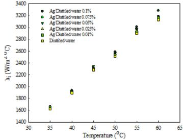
**Fig. 10.** The heat transfer coefficient of distilled- water/silver nanofluid with volume fractions 0.01%, 0.025%, 0.05%, 0.075% and 0.1% compared to the temperature in constant Reynolds number
