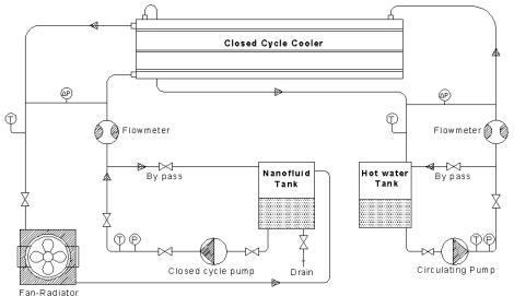
Fig. 3. Experimental closed cycle system
