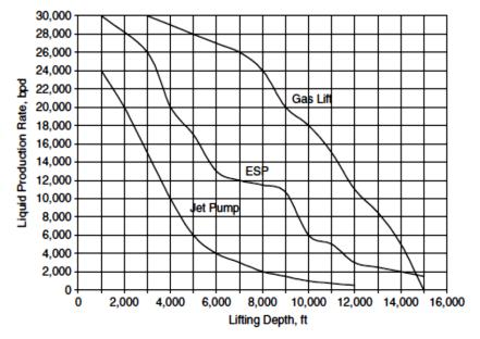
Fig. 1. Comparison of different methods of EOR based on oil liquid rate [3]
