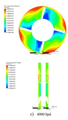
Fig. 11. GVF contour for vortex separator (viscosity: 10 cp, GVF: 30%)
