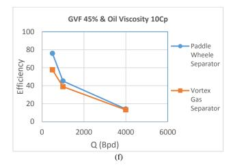
Fig. 9. Effect of GVF and viscosity of paddle wheel and vortex gas separator
