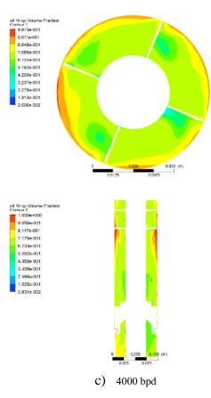
Fig. 10. GVF contour for paddle wheel separator (viscosity: 10 cp, GVF: 30%)
