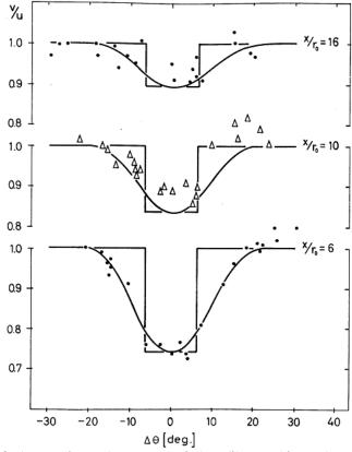
Fig.1. Experimental measured wind profile at turbine wake [15]
