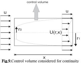
**Fig.9.**Control volume considered for continuity equation
