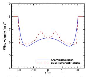
**Fig.10.**Comparison of analytic speed profile with speed profile obtained using BEM method in distance of zero behind wind turbine
