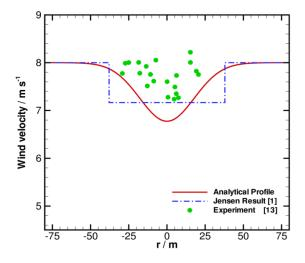
**Fig.13.**Comparison of analytic speed profile with experimental data from Høistrup in distance of 16 times as longer as rotor radius
