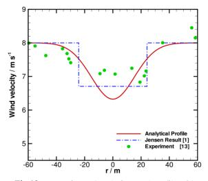
**Fig.12.**Comparison of analytic speed profile with experimental data from Høistrup in distance of 10 times as longer as rotor radius
