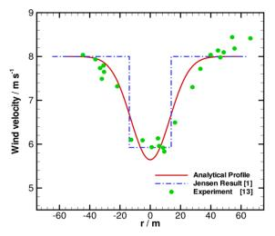
**Fig.11.**Comparison of analytic speed profile with experimental data from Høistrup in distance of 6 times as longer as rotor radius
