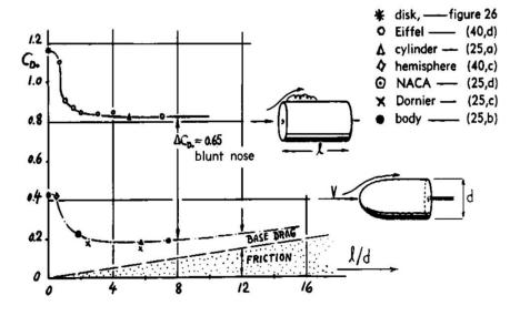
Fig.6. Drag of a blunt cylinder [17]
