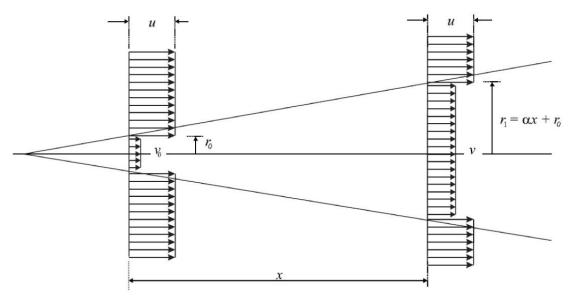
Fig.2. Schematic wake model of Jensen [1]
