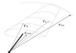
Fig.7.Radial distances of wind turbine blade
