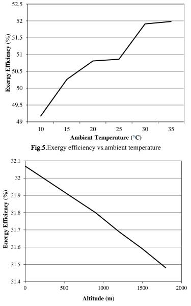
Fig.6.Energy efficiency as a function of altitude
