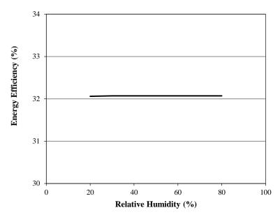
Fig.8.Energy efficiency vs.ambient relative humidity
