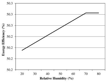
Fig.9.Exergy efficiency vs.ambient relative humidity
