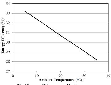
Fig.4.Energy efficiency vs.ambient temperature
