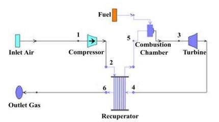
Fig.1.Schematic of recuperated microturbine cycle
