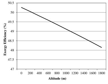
Fig.7.Exergy efficiency as a function of altitude
