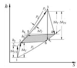
Fig.2. Recuperated gas turbine h-s diagram
