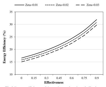
**Fig.3**.Energy efficiency of the cycle as a function of effectiveness
