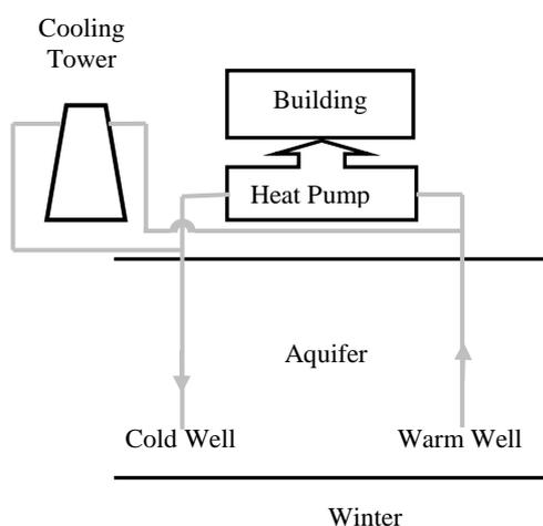
Fig. 2. Combination of ATES with a heat pump for heating and cooling of the buildings
