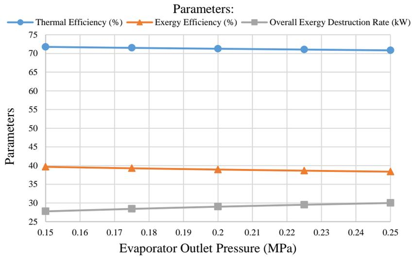
Fig. 3. Effect of the evaporator outlet pressure on the thermal efficiency, exergy efficiency, and overall exergy destruction ratio
