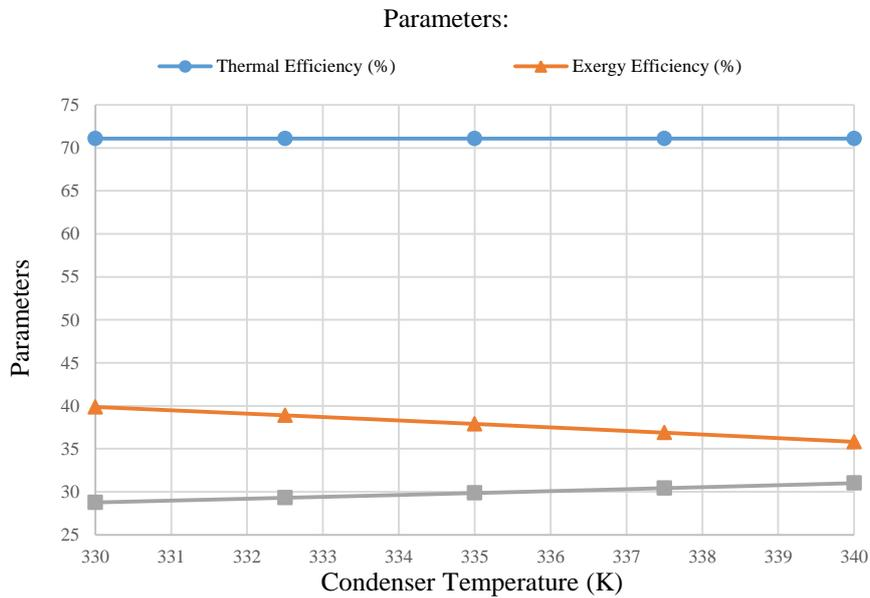
Fig. 5. Effect of the condenser temperature on thermal efficiency, exergy efficiency, and overall exergy destruction ratio
