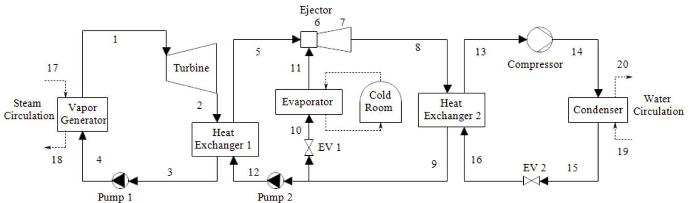
Fig. 1 Schematic of thermodynamic cycle of the proposed CCHP system
