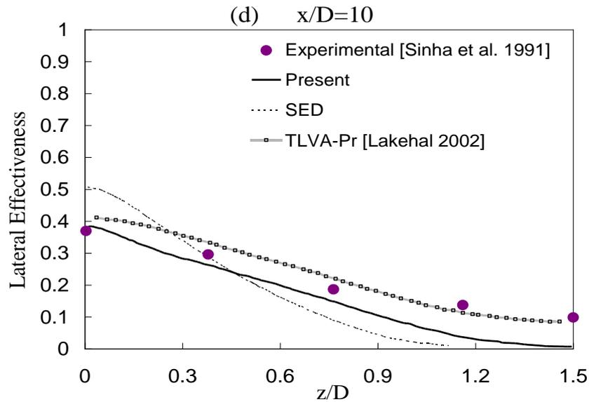
Fig. 11. Spanwise distributions of local film cooling effectiveness.
