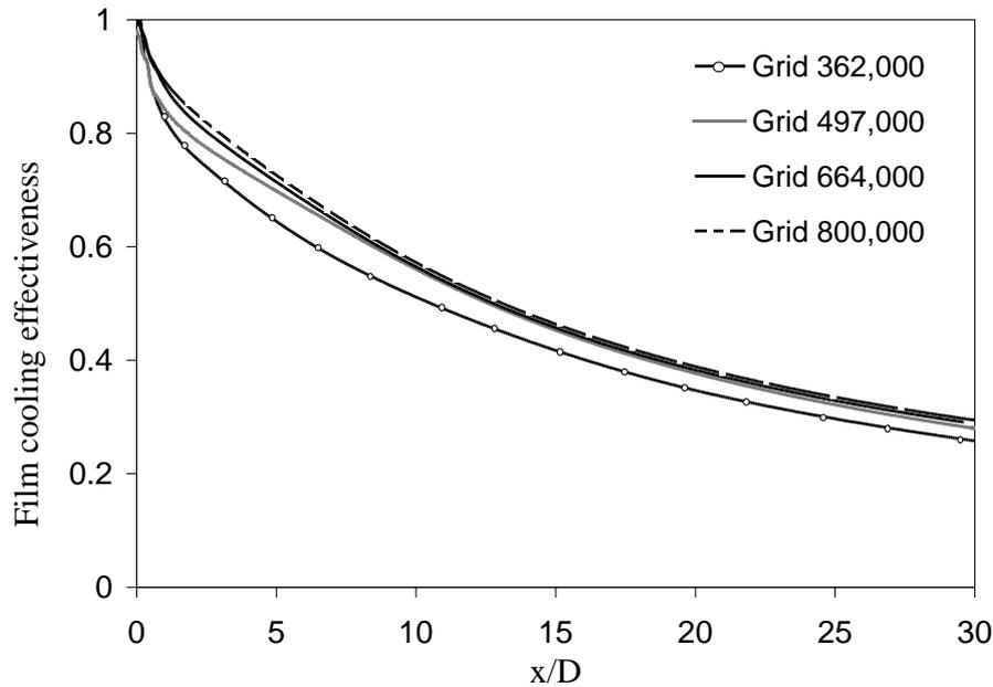
Fig. 3. Effect of grid size on the predicted film cooling effectiveness.
