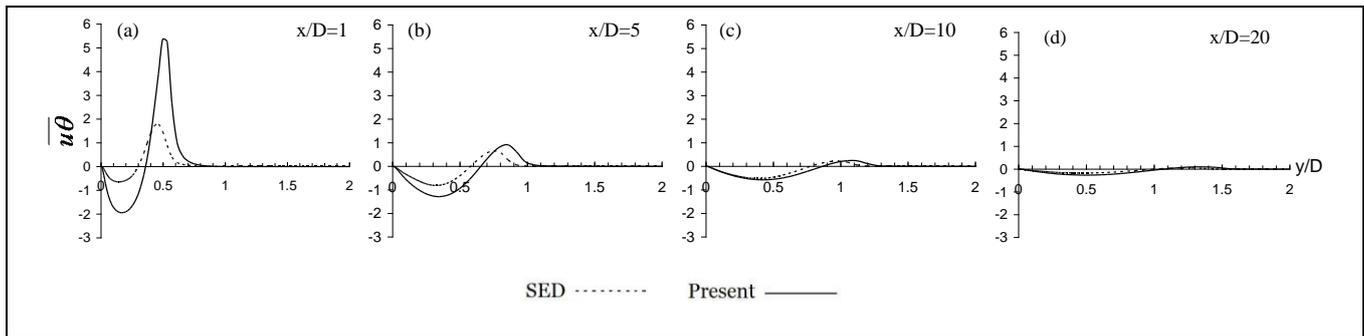
Fig. 8. Streamwise turbulent heat flux distributions at the center-line plane: comparison of SED with the present first-moment closure.
