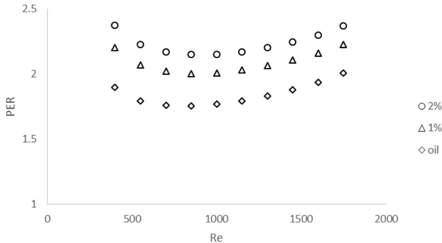
Fig. 12. Comparison of nanofluid efficiency with a base oil in tube AF3
