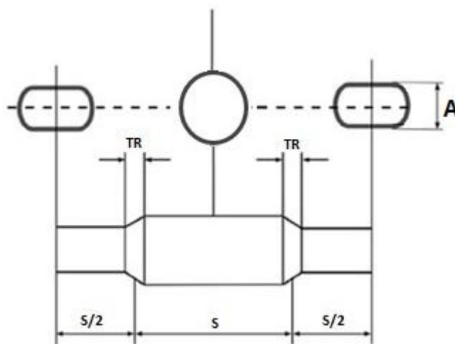
Fig. 4. Schematic of alternating flattened tube
