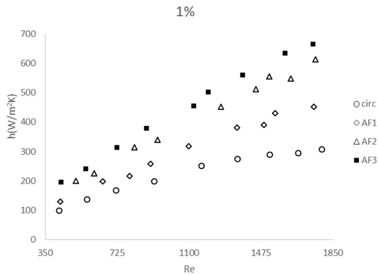
Fig. 7. heat transfer of nanofluid 1% in tubes
