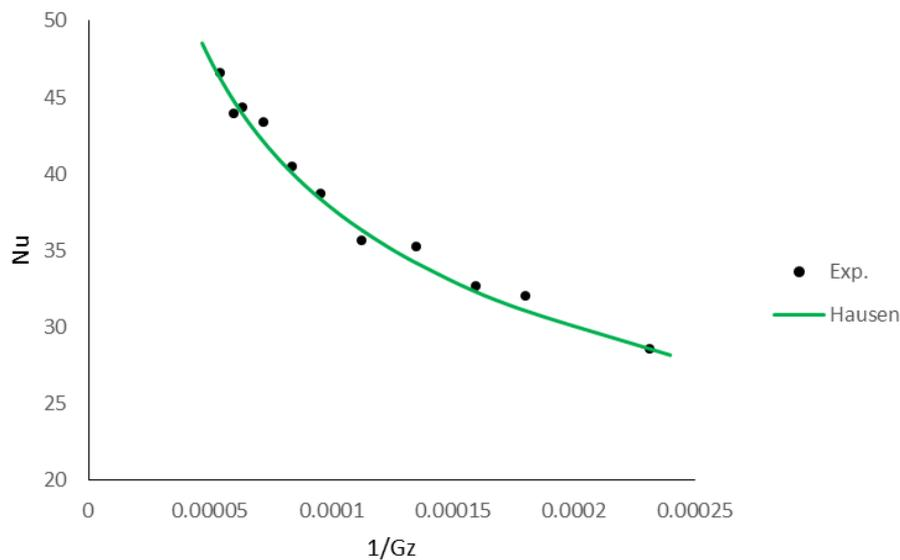
Fig. 2. Comparison of the heat transfer results of the test apparatus with the Hausen equation
