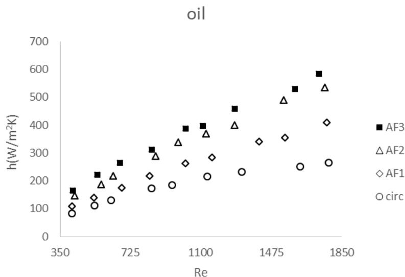
Fig. 5. Heat transfer of base oil in tubes
