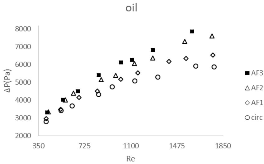
Fig. 6. pressure drop of the Base oil in tubes
