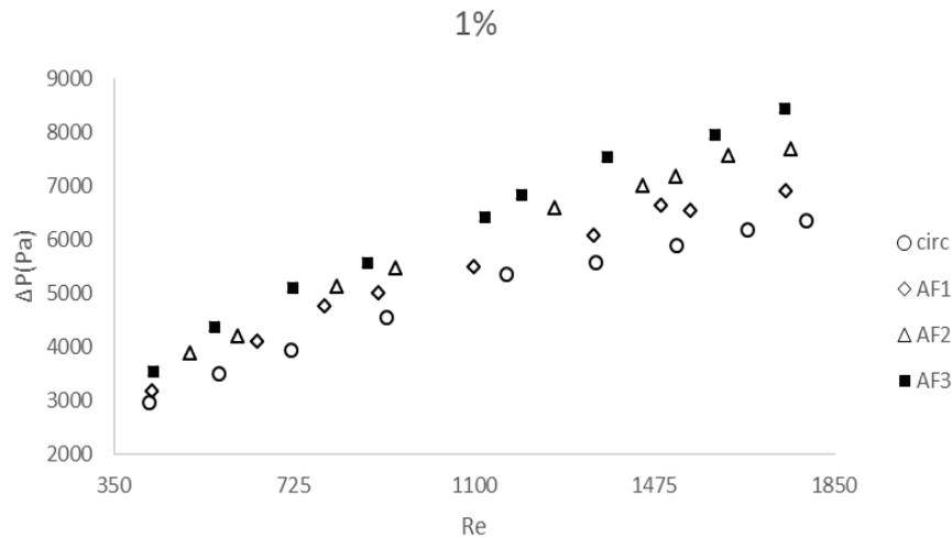
Fig. 9. pressure drop of nanofluid 1% in tubes
