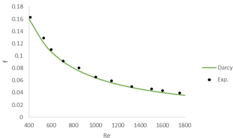
Fig. 3. Comparison of the pressure drop results from the test apparatus with the Darcy equation
