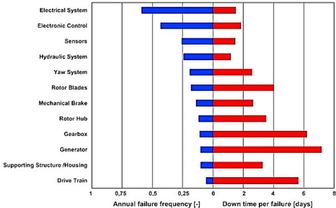
Fig. 1 Annual failure frequency and corresponding downtime for several WT components [3]
