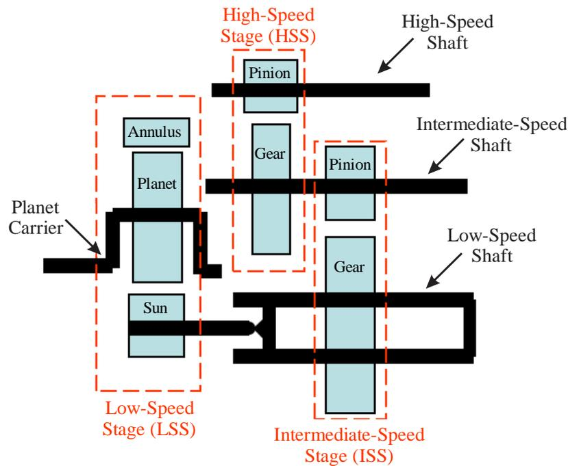
Fig. 4 Test gearbox interior layout [27]
