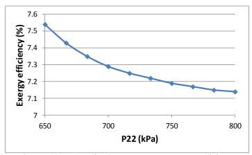
Fig. 4. Effect of turbine inlet pressure on exergy efficiency
