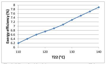
Fig. 3. Effect of turbine inlet temperature on exergy efficiency
