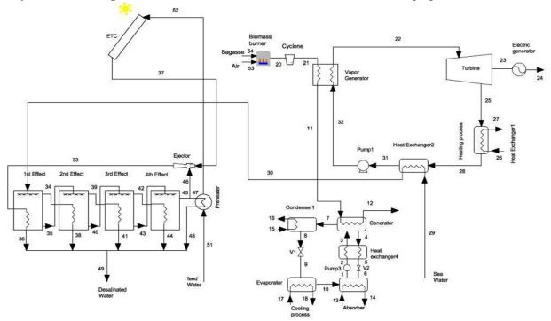
Fig. 1. Schematic of the proposed multigeneration system
