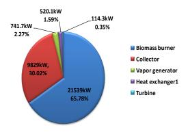
**Fig. 2.** Exergy destruction rate of components of multigeneration system
