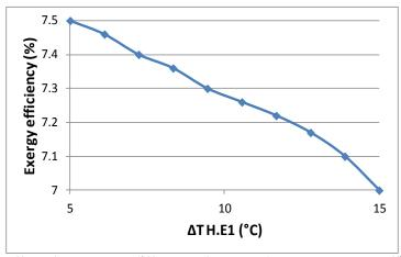
Fig. 5. Effect of temperature difference of Heat Exchanger 1 on exergy efficiency
