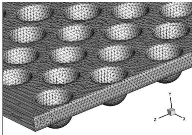
Fig. 2. Schematic of the unstructured mesh
