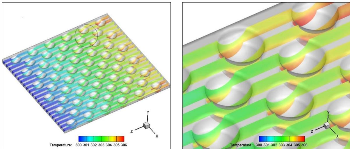
Fig. 5. Contour of temperature distribution at the inlet velocity of 0.75 m/s
