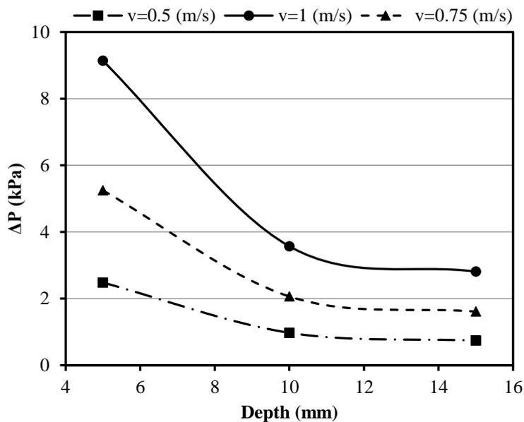
Fig. 7. The effect of Chevrons depth on the pressure drop
