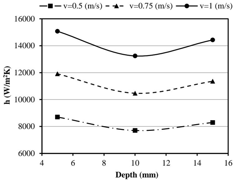
Fig. 6. The effect of Chevrons depth on the convective heat transfer coefficient
