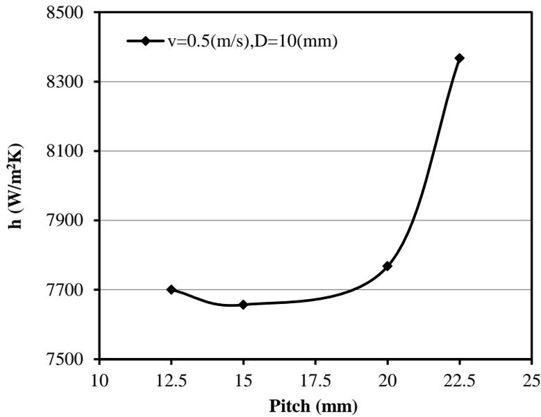
Fig. 8. The effect of Chevrons pitch on the convective heat transfer coefficient
