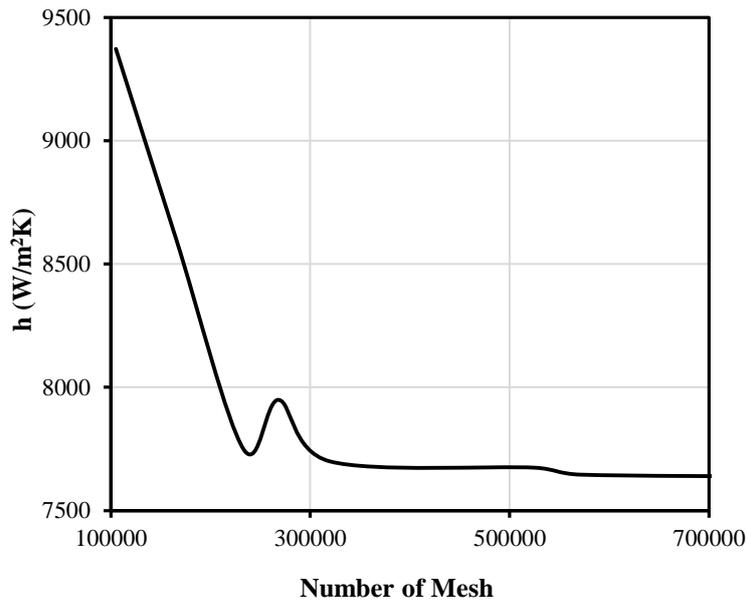
Fig. 3. The effect of the grids number on the convective heat transfer coefficient
