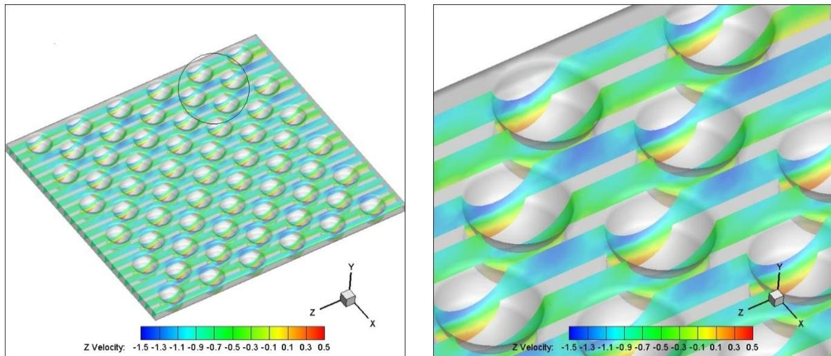
Fig. 4. Contour of velocity distribution at the inlet velocity of 0.75 m/s
