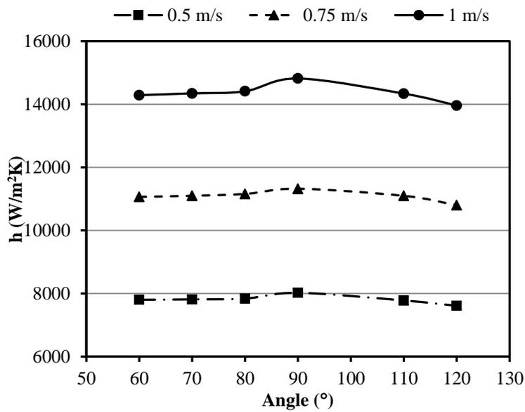
Fig. 10. The effect of Chevrons angle on the convective heat transfer coefficient
