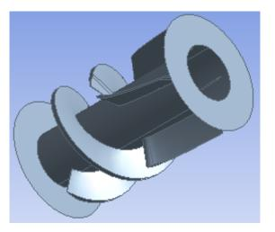
Fig. 2. Paddle wheel separator
