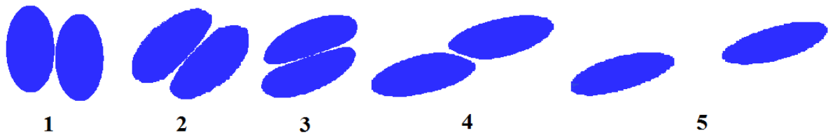
Fig. 4. Sequences (1-5) exhibiting the binary collision of drops in simple shear flow when Ca = 0.2 , offset = 2, and \lambda = \eta = 1 .
