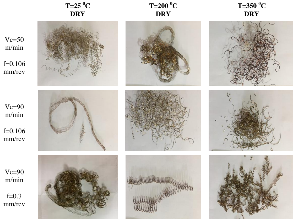
Fig.8. chips obtained from machined specimens under dry condition and different machining parameters
