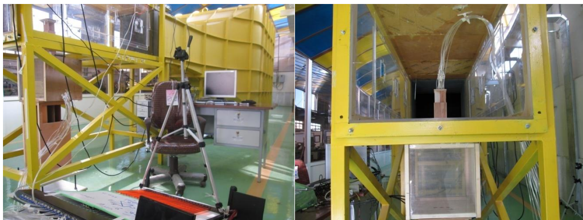
Fig. 2. The wind tunnel and experimental test box.
