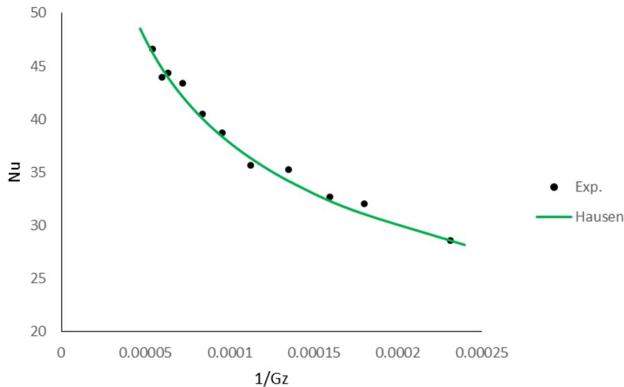
Fig. 2. Comparison of the heat transfer results of the test apparatus with the Hausen equation
