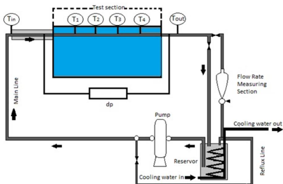
Fig. 1. Schematic of the test apparatus
