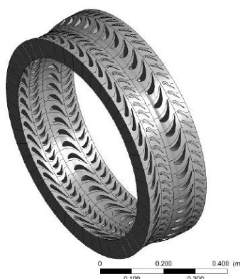
Fig. 2. Three-dimensional geometry of the E3 turbine.
