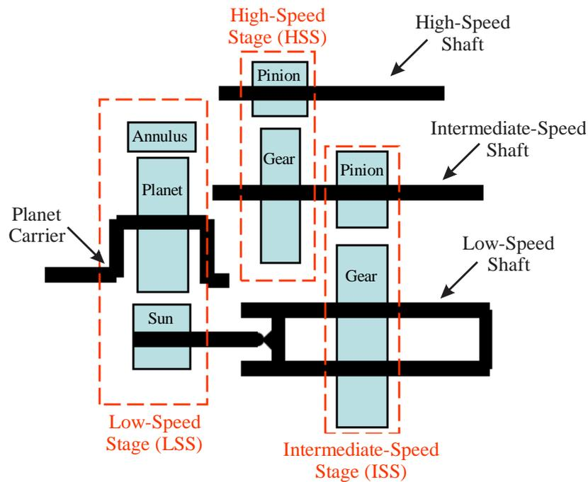
**Fig. 4** Test gearbox interior layout [27]
