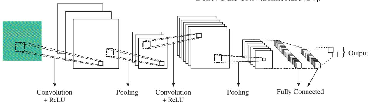
**Fig. 2** convolutional neural network architecture
