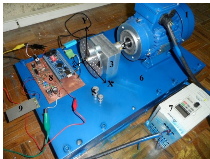
Fig.1. Laboratory system for study of piezoelectric beams 1.Electromotor 2.Shaft 3 Support 4.Disk 5.Mis-alignment mass 6.Chassis 7.Inverter 8. Electrical circuit 9. Piezoelectric beam
